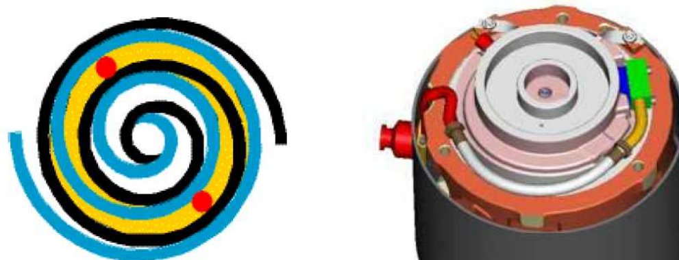
Figure 2: Position of the injection ports in the scroll set and the internal tubing connecting the injection inlet with the scroll set
